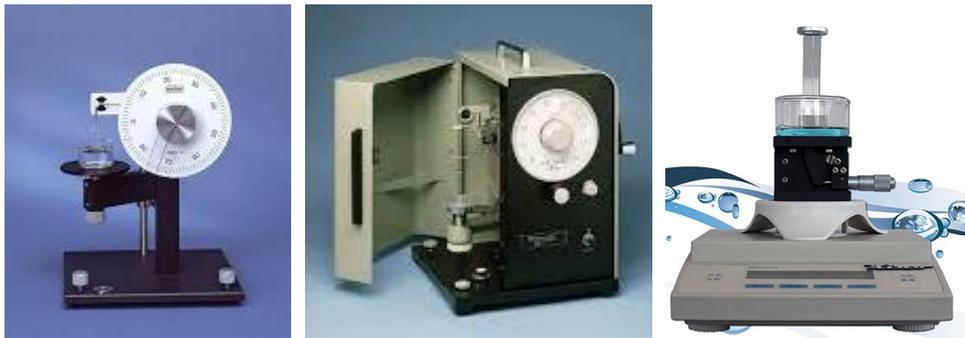
Cheaper tensiometer: left one is Classical Du Noüy ring Tensiometer used torsion wire sensor, middle one is tensiometer made by fisher and right one is tensiometer model A3 made by KINO which used balance as sensor. Please be noted that KINO is only one that provides tensiometer at price about 1500USD using balance.
